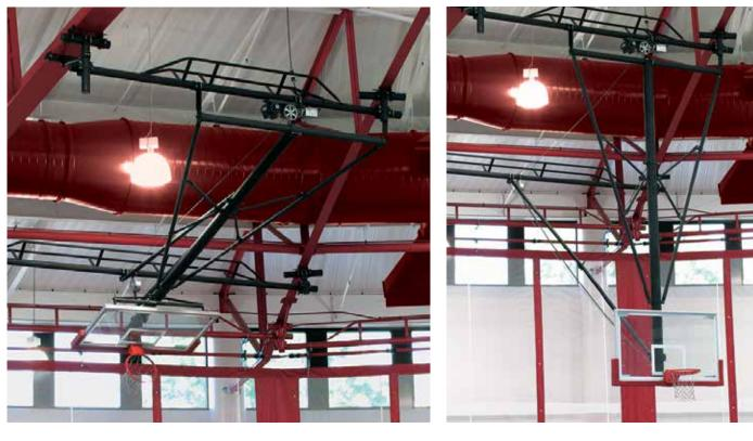
Nothing in front of the backboard makes TB-25 Basketball Backstop preferred by coaches. Backstops are custom designed so the lateral sway brace intersects the main mast at approximately 54" (1.37 m) above the goal and 18" (46 cm) above the backboard; to ensure maximum rigidity.
